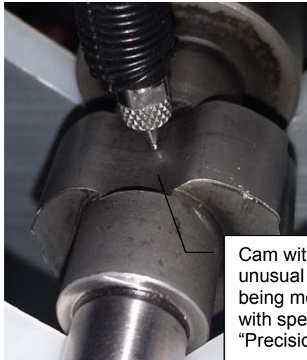
Figure 9.4 Measure Anything Option To Measure Unusual Cams
