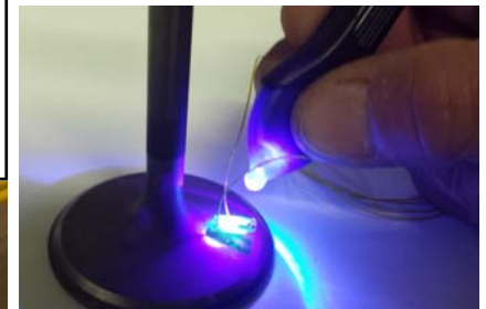
Fig 3 Attaching Remote Velocity Tip with UV cured glue
